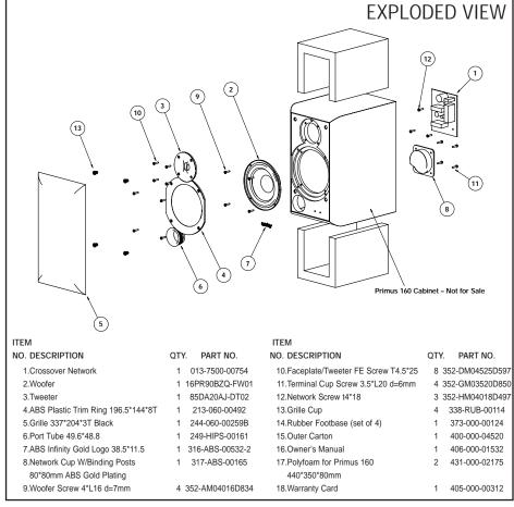
Note: A Phillips screwdriver and "Torx" bit screwdriver T20 size are required to service this product
